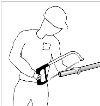
10 - Adjust last section by sawing swagged extra
