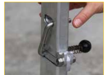
4. Engage the handle in the lock by releasing the locking handle (the lock has notches) to lock the upright completely, then push the handle outwards until it reaches the last notch. The system is now fully locked.
